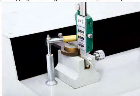
lapping measuring surfaces of caliper lower jaws
